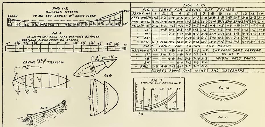
and the deck beam fastened to the ends of the frames. Before putting in the screws lay the parts together and check them for width and height. You can lay out a baseline and centerline on the floor to aid in this work.
