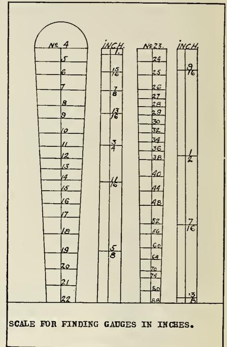
scale. At once we see that our gauge is between 1/2 and 9/16 of an inch in diameter. On closer inspection we see that our 28 ga. line divides the distance between 1/2 and 9/16 approximately 3/5ths of the distance above the 1/2. This space between 1/2 and 9/16 represents 1/16 of an inch.  $3/5 \times 1/16 = 3/80$ ; therefore 1/2 plus 3/80 = 43/80 inches, which is the diameter of our bore. Reduced to a decimal fraction 43/80 is equal to .54 (This is very close to the true value, .55).
