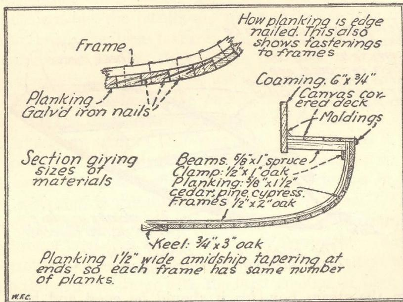
the stern and also the bow. By making these divisions equal on each mold, as well as the bow and stern, the planks will fit well and there will be no feather edges. Of course, the planks for one side should be made in duplicate for the other, and in the drawing, the planking is shown as being  $1\frac{1}{2}$ " wide amidships. This may be varied slightly to suit local conditions, but if the wood is too wide, it will not lie up flush against the frames or molds.
