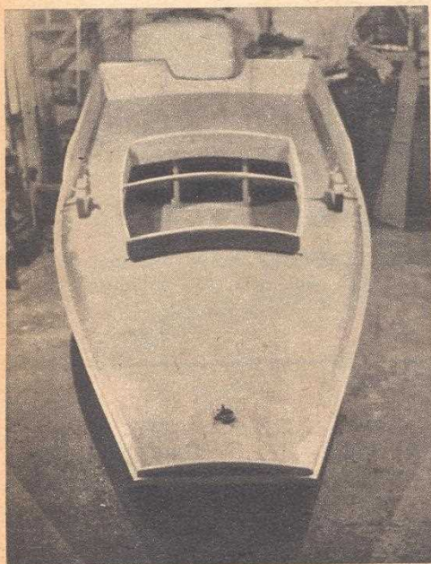
AFTER HULL is fibreglassed, install bottom runners, cockpit coamings and rack boards.
