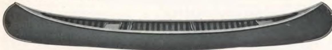
This is an exceptionally high grade canoe. An easy paddling canoe with good capacity and a wide flat floor that makes it steady and safe. Built of selected materials, and with decks, seats and thwarts of mahogany, hardwood outwales outside stems, and  $\frac{7}{8}$ " keel, it is very attractive in appearance. Stocked in one size only, and in Red or Green enamel finish.
