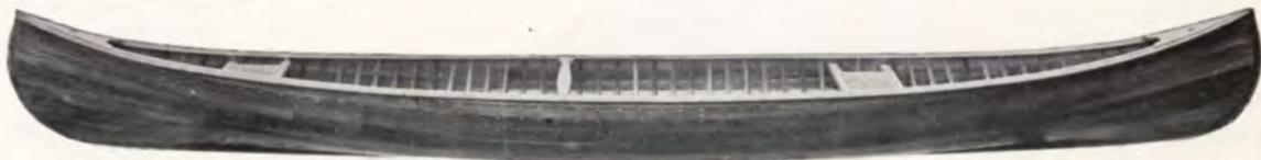
**The "RIVERDALE"** (No. P404) Length 16 feet. Beam 31 inches. Depth 12 inches. Weight 62 lbs.
