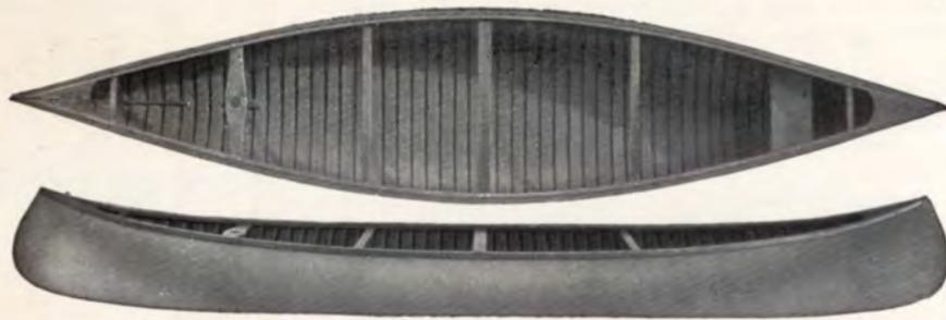
Canoes Nos. 670, 671 and 572 do not tumble in on the sides like other canoes. The sides are straight or flare out, making them drier in rough water.
