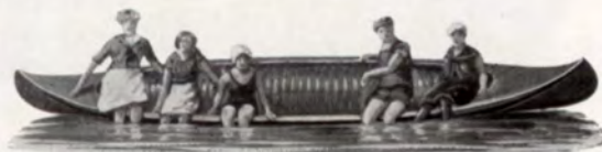
The "SPONSONS" support the weight and keep the gunwale above water.
