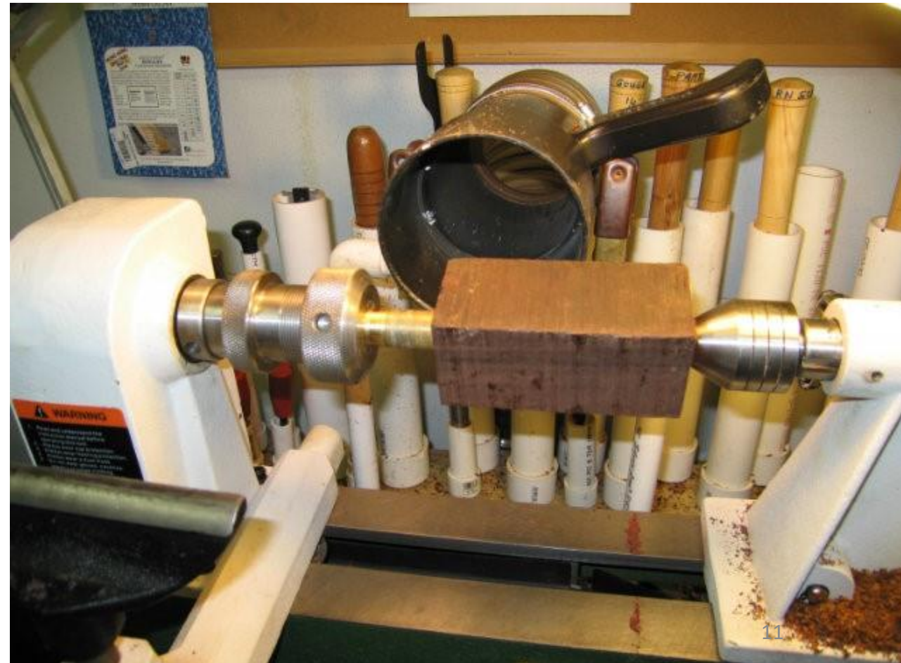
Call blank mounted on the expanding mandrel
