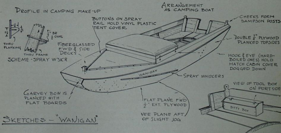
enlarged beam to the floor area between chines, tilted the lath to proper angles for stiffening the hull up under burden, and, transferring the resulting measurements to my notebook, sketched the profile and deck plan of the boat presented here.
