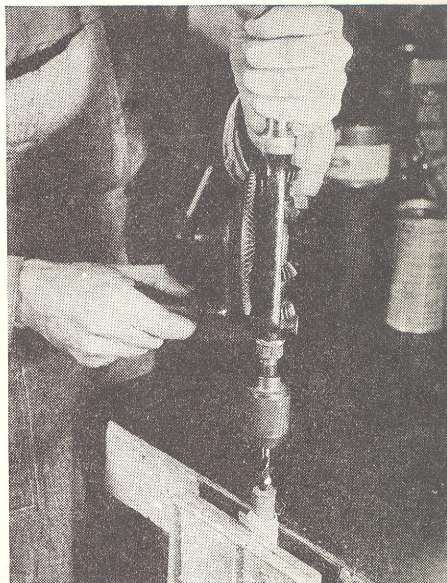
Drilling the hole in the shaped blank. A twist drill (like that shown) often cuts end grain more easily than an ordinary auger bit
